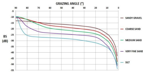
Figure 2 theoretical BS curves as a function of grazing angle for several types of bottom floor (figure from GeoHab workgroup report may 2015, data source University of Washington Applied physics lab)
