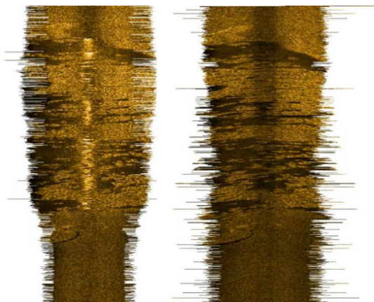
Figure 3 left : waterfall of BS measurement from transverse swath, right : BS from transverse swath steered 20° forward
