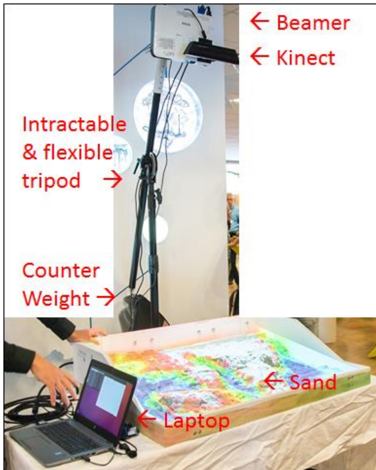
Figure 1: Sandbox-FM setup illustrating the connection between the different components
